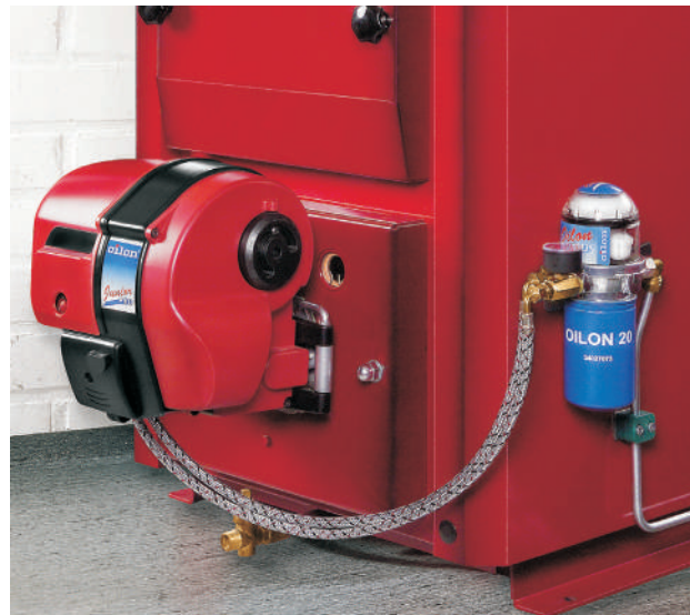
Oilon Plus is equipped with vacuum gauge and shut-off valve. When vacuum gauge indicator is on the red area, the filter has to be changed.
